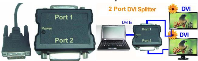
The 2 Port DVI Splitter can repeat one DVI signal to 2 Port DVI signal sets support up to 2 different DVI display terminals. Based on Cleared Edge technology, it supports up to 3.4Gbps data rate per channel, compliant with the DVI1.0 specification. This Splitter supports integrates EDID.
