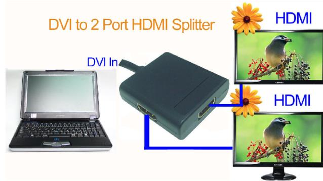
The DVI to 2 ports HDMI Splitter can repeat one DVI signal to 2 HDMI signal sets support up to 2 different HDMI display terminals. Based on Cleared Edge technology, it supports up to 3.4Gbps data rate per channel, compliant with the DVI1.0 & HDMI 1.3 specification. This Splitter supports integrates EDID.
