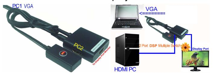
VGA (PC1) +HDMI (PC2) to Display Port Monitor, with control box (The control box lights to select PC2).
