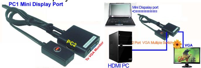
Mini Display Port (PC1) +HDMI (PC2) to VGA Monitor Switch, with control box (The control box lights to select PC2).
