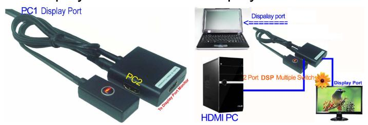
Display Port (PC1) +HDMI (PC2) to Display Port Monitor, with control box (The control box lights to select PC2).
