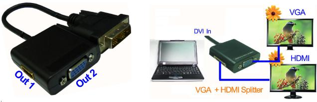
The DVI to HDMI & VGA Splitter can converter one DVI signal to HDMI & VGA signal sets support up to 2 different HDMI & VGA display terminals. Based on Cleared Edge technology, it supports up to 3.4Gbps data rate per channel, compliant with the HDMI1.4 specification. This Splitter supports integrates EDID.
