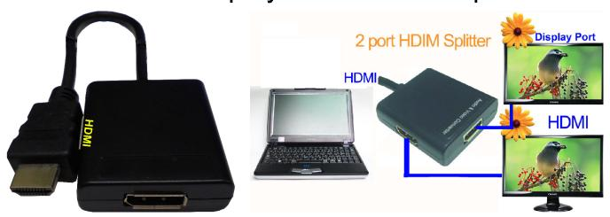
The HDMI to Display Port & HDMI Splitter can converter one HDMI signal to Display Port & HDMI signal sets support up to 2 different Display Port & HDMI display terminals. Based on Cleared Edge technology, it supports up to 3.4Gbps data rate per channel, compliant with the HDMI 1.4 specification. This Splitter supports EDID of self.
