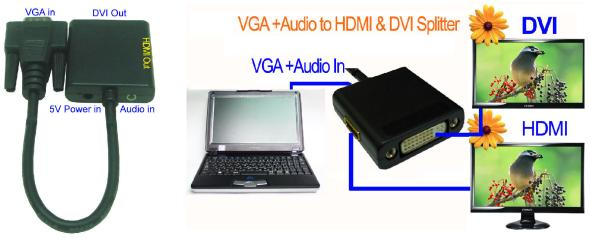
The VGA+ Audio to HDMI & DVI Splitter can converter one Mini VGA & Audio signal to HDMI & DVI signal sets support up to 2 different HDMI & DVI display terminals. Based on Cleared Edge technology, it supports up to 3.4Gbps data rate per channel, compliant with the HDMI 1.3 specification. This Splitter supports integrates EDID.
