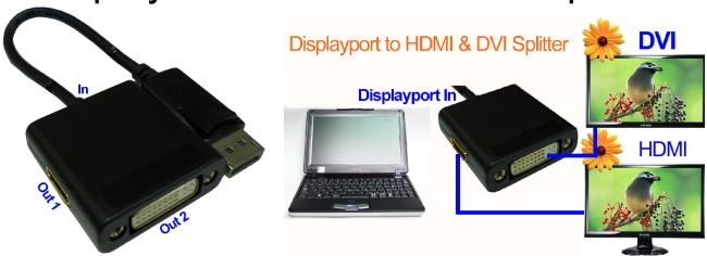
The Display port to HDMI & DVI Splitter can converter one Display port signal to HDMI & DVI signal sets support up to 2 different HDMI & DVI display terminals. Based on Cleared Edge technology, it supports up to 3.4Gbps data rate per channel, compliant with the Display port 1.2 & HDMI 1.3 /DVI1.0 specification. This Splitter supports integrates EDID.
