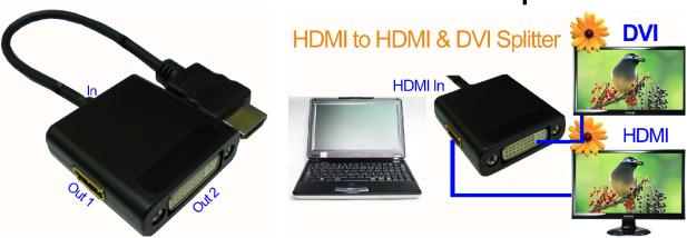
The HDMII to HDMI & DVI Splitter can repeat one HDMI signal to HDMI & DVI signal sets support up to 2 different HDMI & DVI display terminals. Based on Cleared Edge technology, it supports up to 3.4Gbps data rate per channel, compliant with the DVI1.0 & HDMI 1.4 specification. This Splitter supports integrates EDID.
