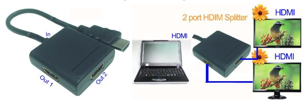
The 2 ports HDMI Splitter can repeat one HDMI signal to 2 HDMI signal sets support up to 2 different HDMI display terminals. Based on Cleared Edge technology, it supports up to 3.4Gbps data rate per channel, compliant with the HDMI 1.4 specification. This Splitter supports integrates EDID.
